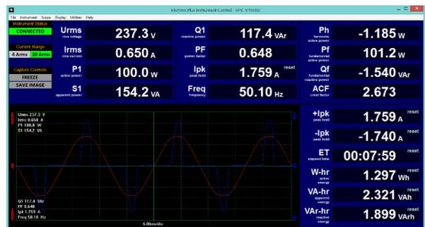
EPIC software from Electron Plus is free-to-use software that connects all our instruments, the CPA100 module within EPIC is designed to present all key measurement data to the user as cleanly as possible, simple to understand menus and intuitive features on the single page layout reduce the learning curve associated with a new instrument and reduces errors in measurement setup.
